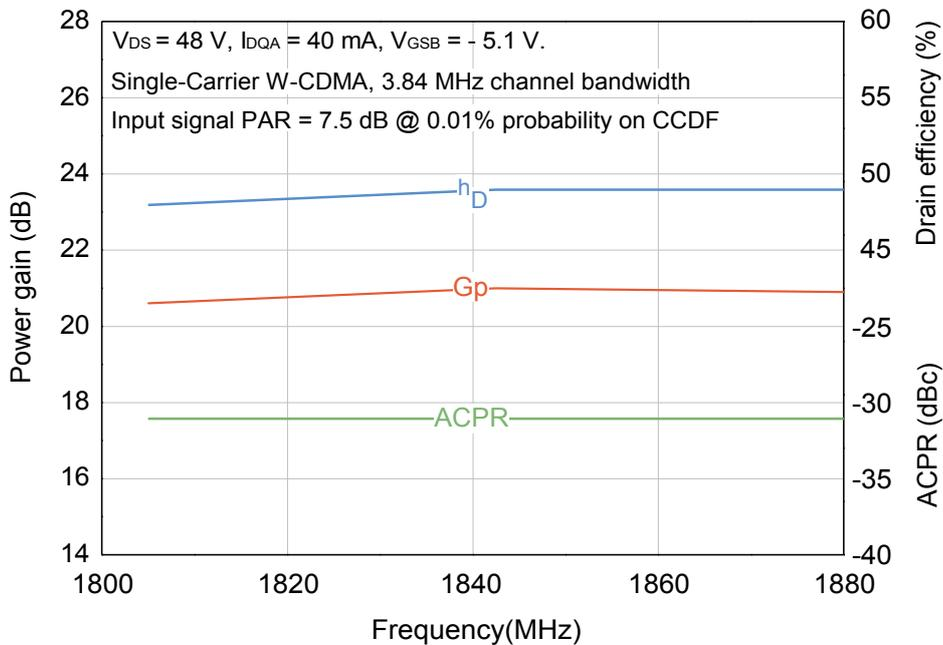
Fig 3. Power gain, Drain efficiency, ACPR vs. Frequency
