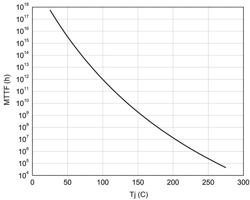
Fig 5. Median lifetime vs. channel temperature
