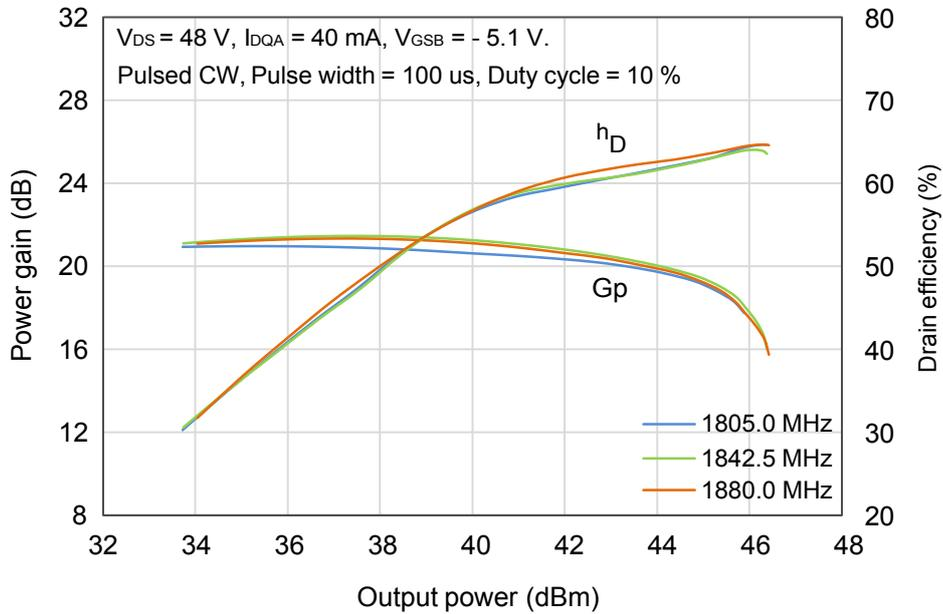
Fig 2. Power gain, Drain efficiency vs. Pulse output power
