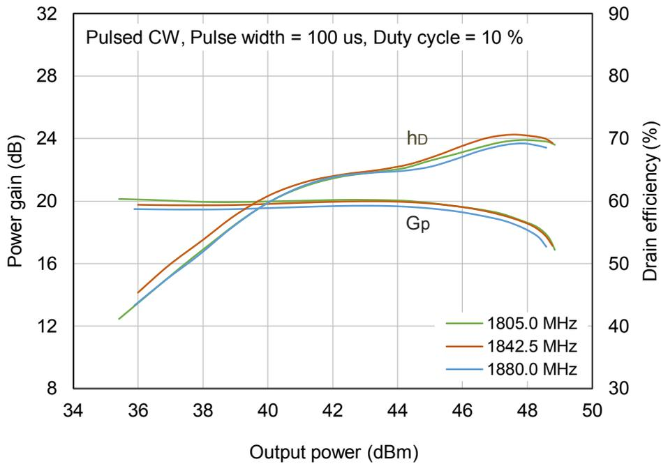
Fig 2. Power gain, Drain efficiency vs. Pulse output power
