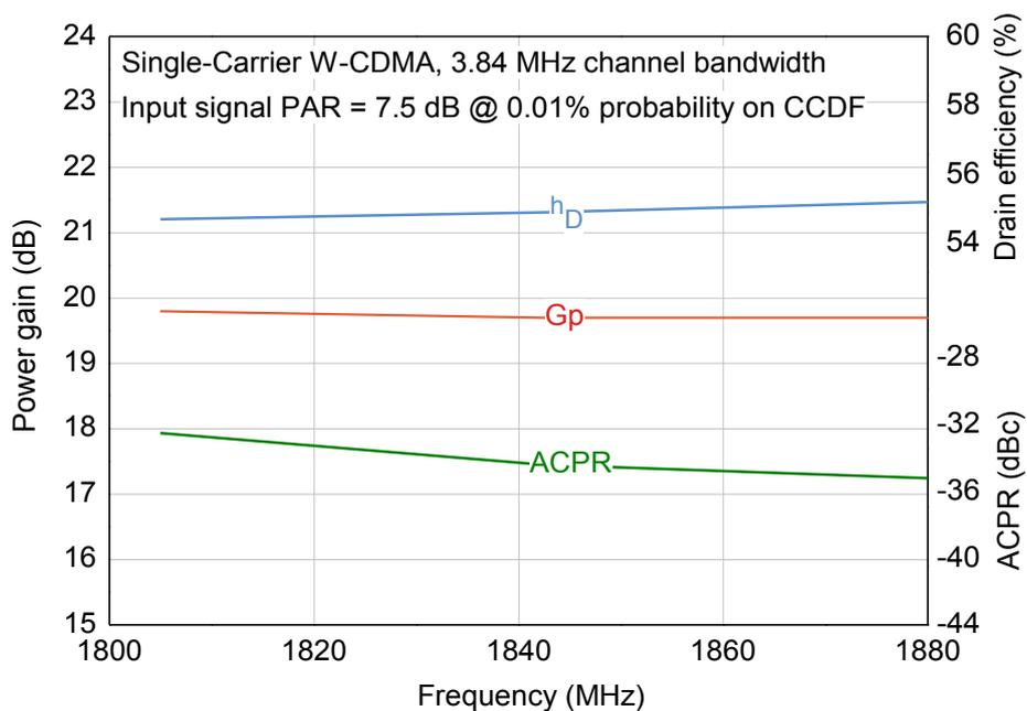
Fig 3. Power gain, Drain efficiency, ACPR vs. Frequency
